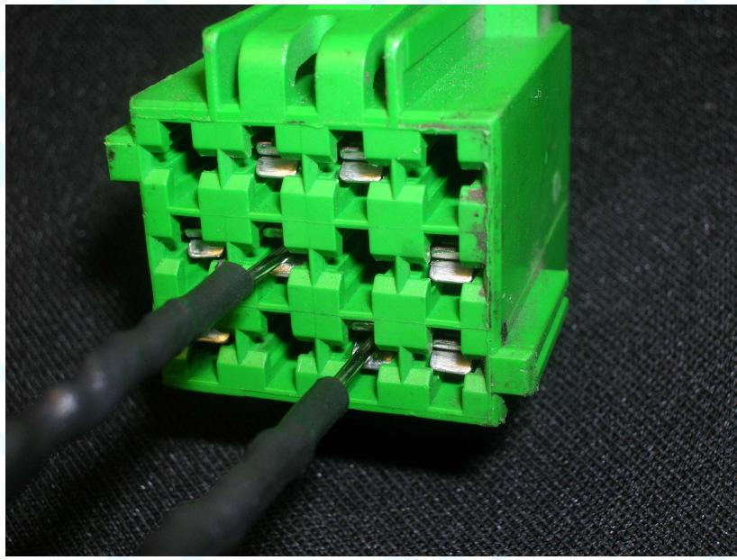
**Plug with 12 pins, heads of the cables
