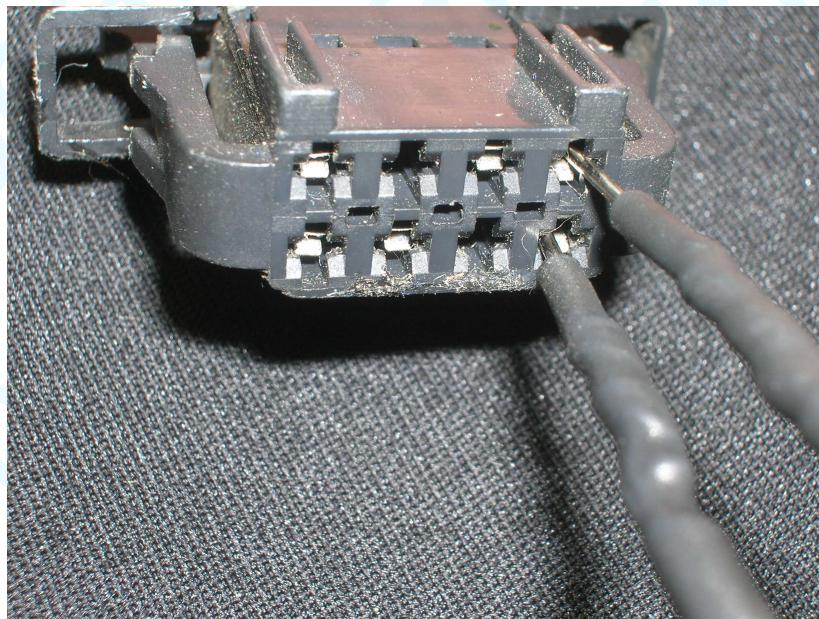
**Plug with 8 pins, heads of the cables
